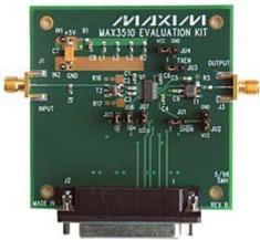
Objective: To complete a set of harmonic distortion tests for MAX3510, from 15MHz to 55MHz (extended band).
